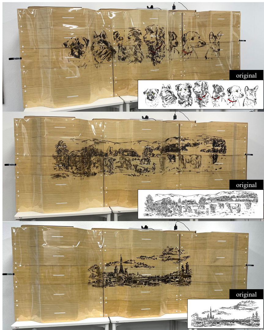
Fig. 12. Robotic drawing results: Dogs, Farm, Paris, from top to bottom. Original vector graphics image and the images drawn on a physical curved surface.
