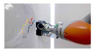
Fig. 5. Force (f) is generated by the impedance-controlled manipulator. The black line represents an expected physical spline curve with its set of control points (blue dots), and the white dotted line represents a virtual spline curve, consists of the set of underestimated target positions (yellow dots).
